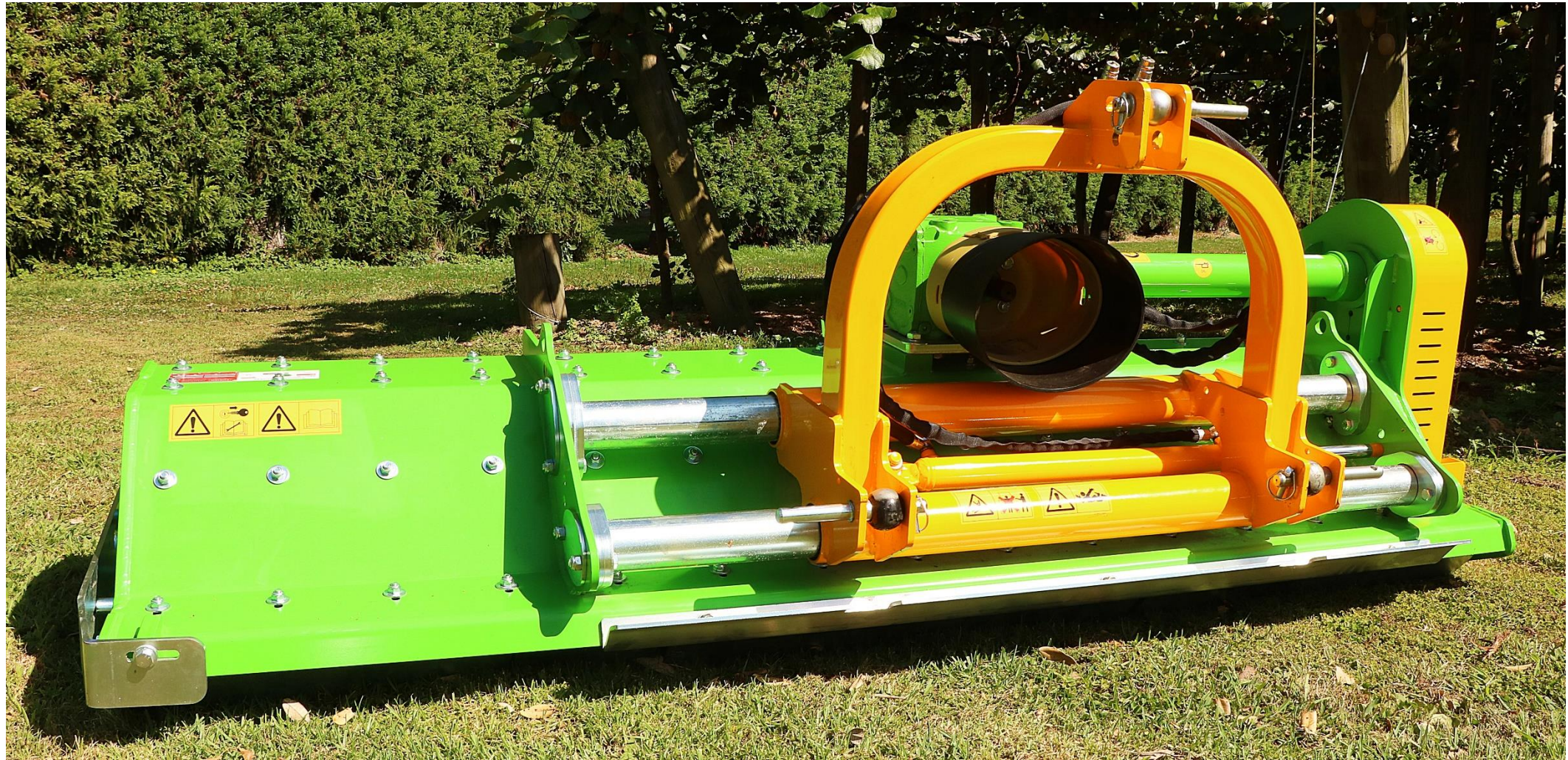
Double replaceable bolted inner skin & Hydraulic side shift standard features.
