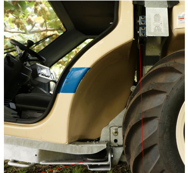
Air Bag suspension on all four corners of the cab.
