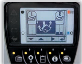
Max. Oil Flow Setting (AUX1 and AUX2)
