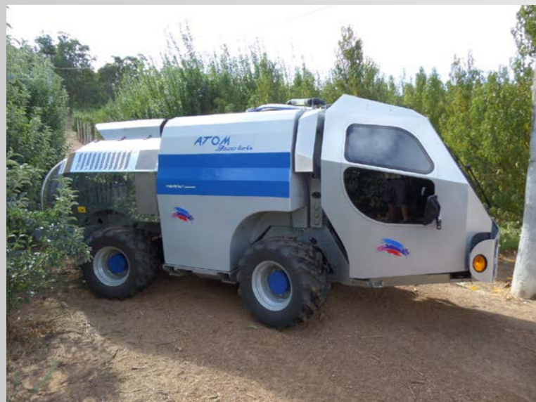
Cabin airbag suspension system over chassis hydraulic suspension system giving the machine a dream like ride. Machine height and ground clearance can be adjusted instantly and are electronically controlled.
