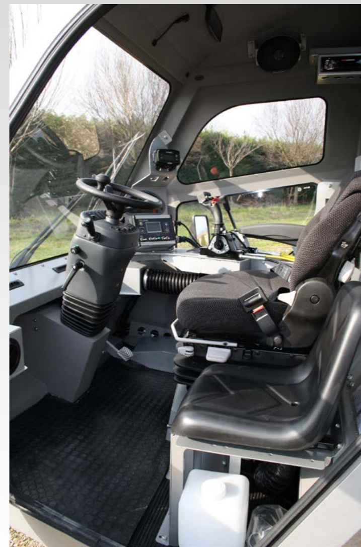
Large roomy cab, fully stainless steel, giving top level of comfort. Superb visibility. Large pneumatic seat with automatic weight adjustment. Wide adjustable passenger seat. High power air conditioning and heating.
