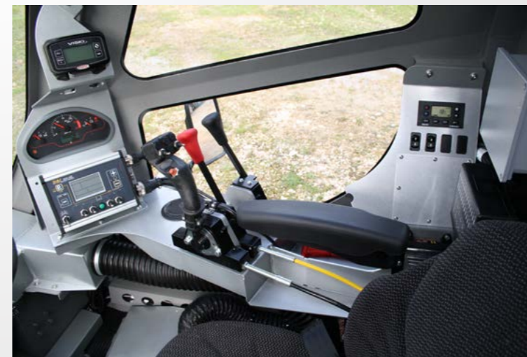
Large roomy cab, fully stainless steel, giving top level of comfort. Superb visibility. Large pneumatic seat with automatic weight adjustment. Wide adjustable passenger seat. High power air conditioning and heating.
