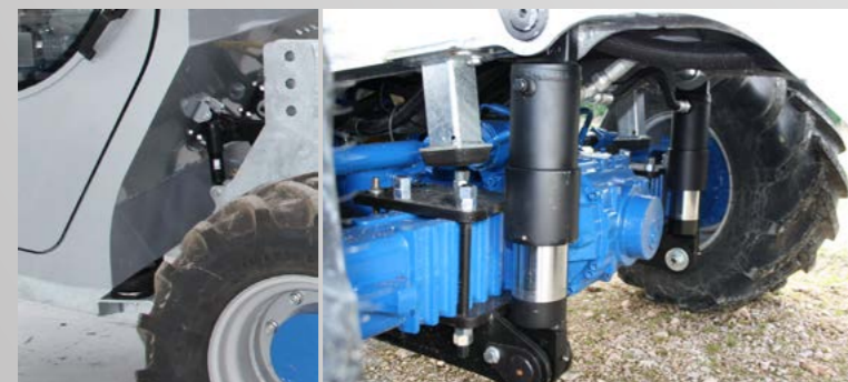
3 modes hydraulic steer: 2 wheel steer, 4 wheel steer, 4 wheel steer crab.
