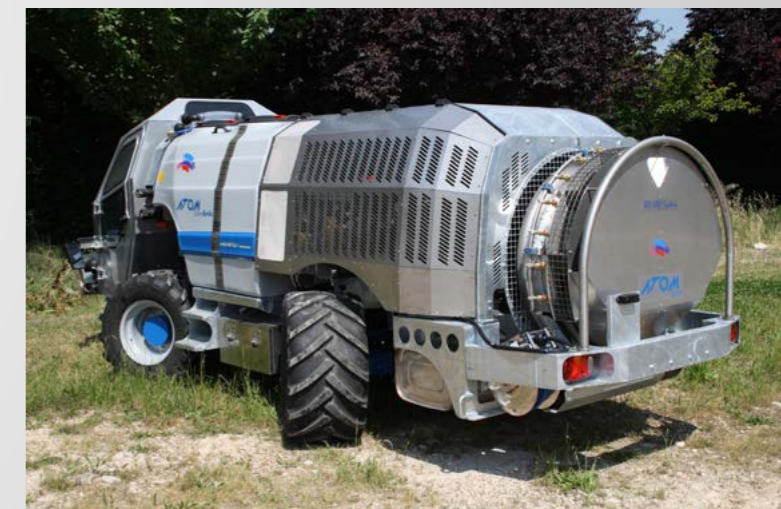
Back hose reel with hand gun. Front and rear auxiliary LED work lights.
