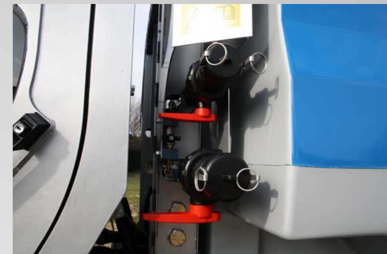
Low tank fill-up points. Venturi chemicals suction system.
