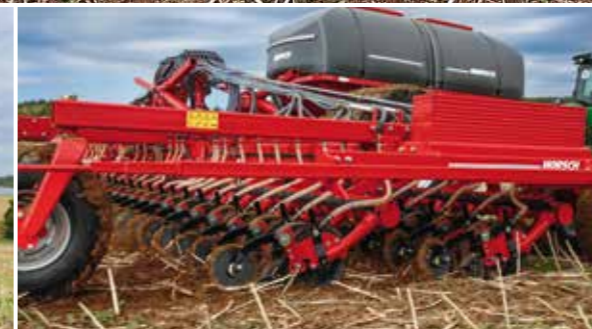
2-bar coulters design for maximum clearance
