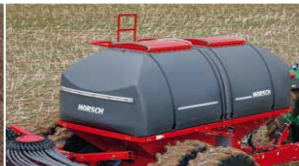
Capacity of 12 000 litre with a 50/50 split hoppers
