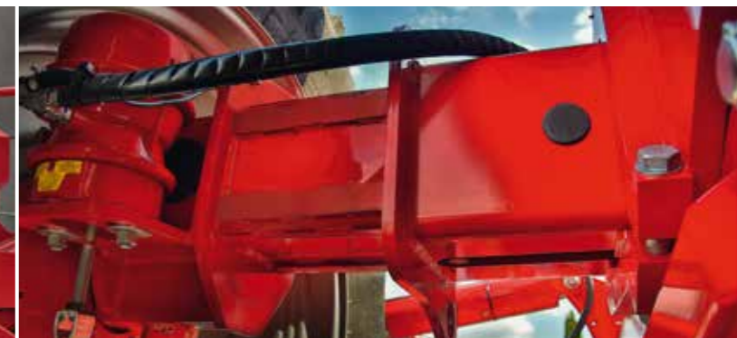
Standard telescopic axle Compact transport width; reduction of the track pressure behind the tractor track
