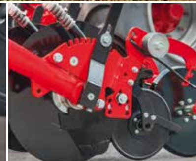
Fine adjustment of the sowing depth
