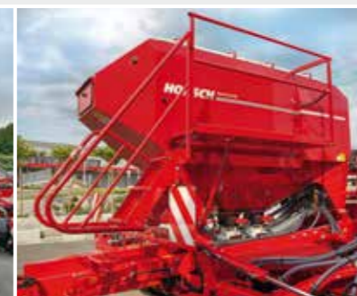
Double hopper 5 000 litre; partition 40/60
