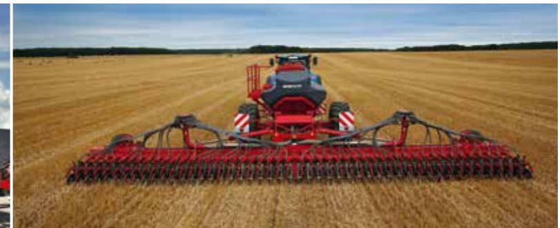
Hydraulic weight transfer from the seed waggon to the coulter frame: Regularly high coulter pressure over the whole working width.
