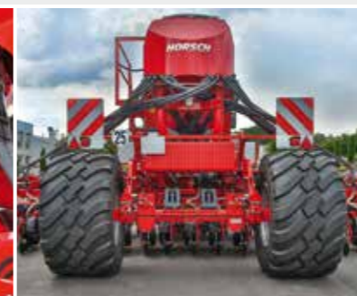
Optional: tyres 710/50–26.5 for maximum contact area
