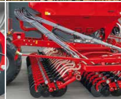
Hydraulic coulters pressure with central adjustment
