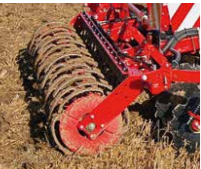
RollFlex packer for a deep consolidation leaving a loose surface
