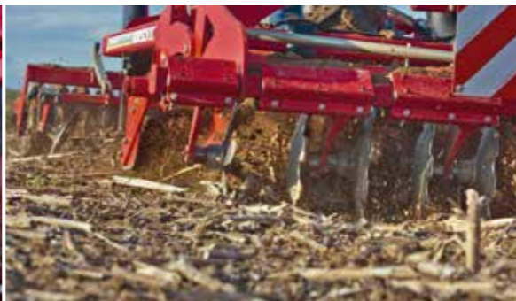
DiscSystem for intensive shallow mixing
