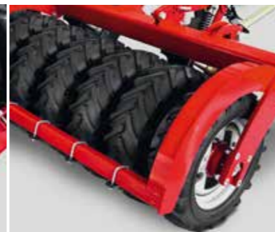
Tyre packer with AS-profile for all-over consolidation
