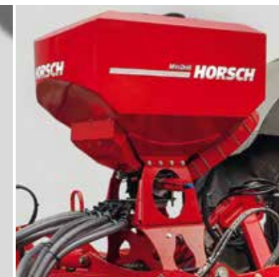
MiniDrill with a hopper capacity of 400 litres
