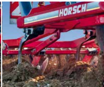
TerraGrip tines with LD coulters for deep loosening of the soil
