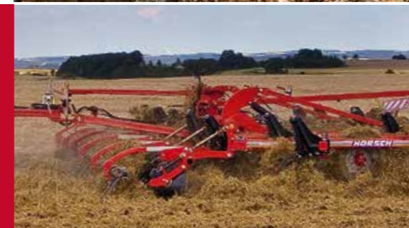
A 1-row levelling disc system and a following harrow are also available instead of a 3-row harrow.
