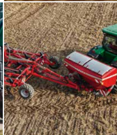
The design of the Partner HT allows for tight turning on the headlands.
