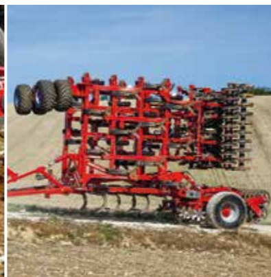
3 m transport width for the Terrano 12 FM
