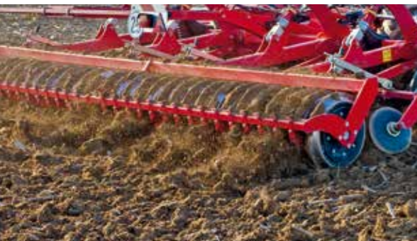
SteelDisc packer for optimum consolidation also on heavy soils
