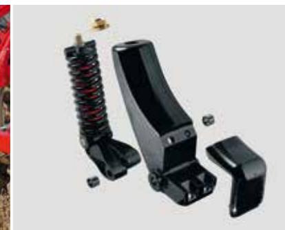
TerraGrip shanks trip height 30 cm, release force 500 kg, maintenance-free
