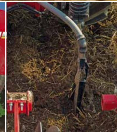
TerraGrip tine with piping and adjustment of the placement depth of the fertiliser depot without tools
