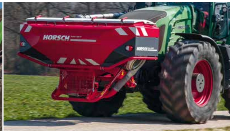
Pressurised hopper with a capacity of 1 600 litre
