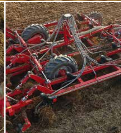
Terrano FM with distribution tower and piping for fertiliser placement
