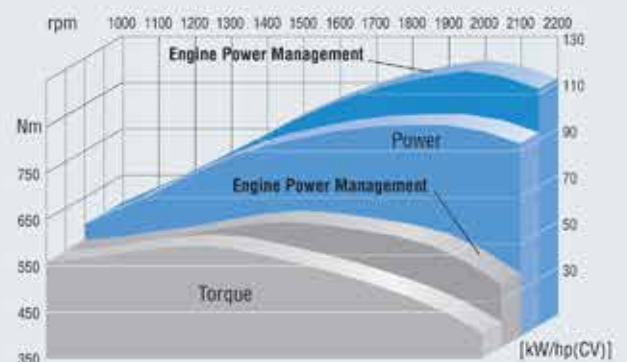
T6050 ELITE POWER & TORQUE CURVES
