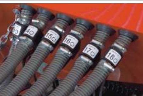
Robust control sensors for seed and fertiliser
