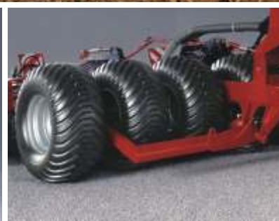
Tyres Optional: eightfold tyres for the complete working width of 6 m.
