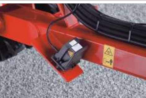
Radar sensor Electronic speed sensor without wheelspin
