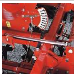
Easy working depth adjustment Hydraulic adjustability during operation
