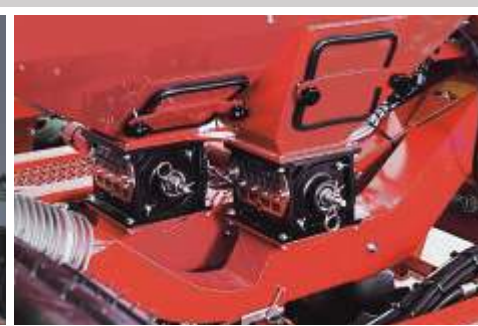
Two identical metering units Precise metering of seeds and fertiliser
