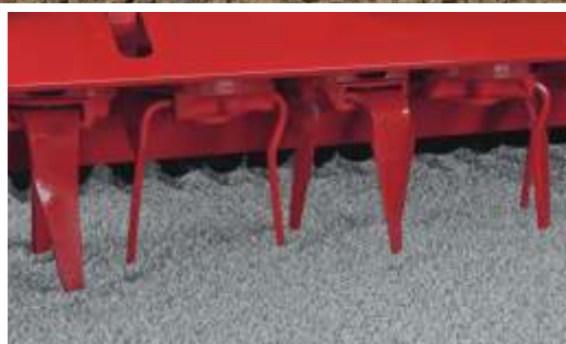
Rotary harrow Drags itself into the soil and constantly maintains the adjusted working depth.
