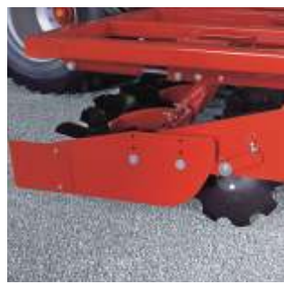
Adjustable side plates Ensures even levelling between passes
