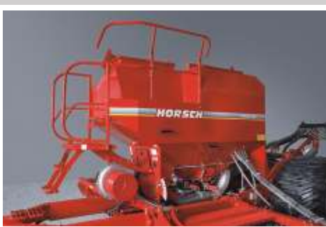
Large double tank Up to 7000 l capacity, 40 / 60 seed / fertiliser
