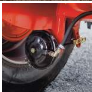
Braking system Pronto AS Dual cycle air brake system, safer road transport
