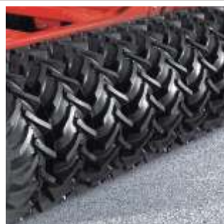
Large tyre diameter (780 mm) Reduces draft requirement
