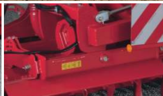
3 m segments of the rotary harrow are oscillatingly suspended for an optimum soil adjustment.
