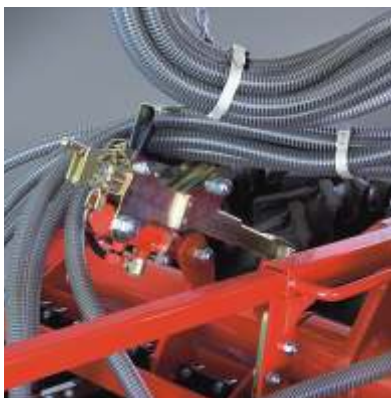
Hydraulic coultter pressure adjustment
