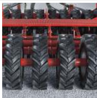
Effective tyre packing system Optimised AS thread for even consolidation
