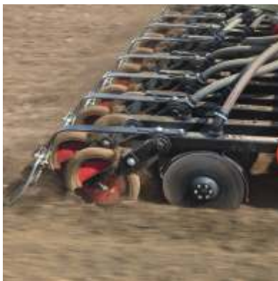
Turbo Disc coulters Precise seed placement at high speed
