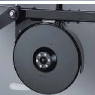
Double disc coupler Straight discs with inner maintenance-free bearings
