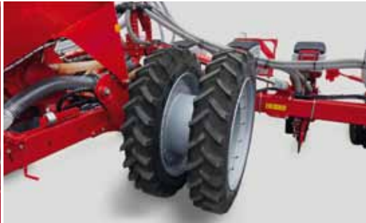
Optional: twin tyres 230/95 R 32 Maestro CC . The seed furrow is exactly between the tyres
