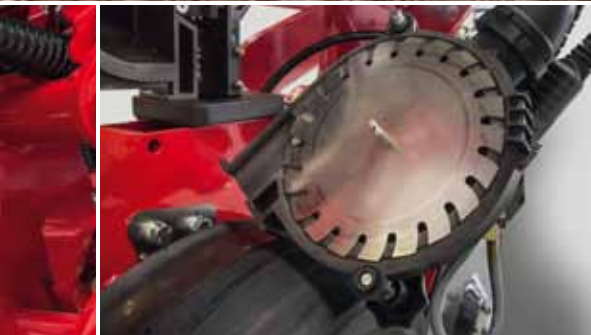
The new metering disc of the Maestro with open grooves.
