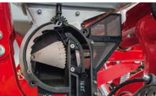
The adjustable scraper transports the grain into the fall sluice without any disturbing centrifugal forces.
