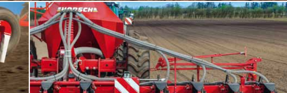
Seed wagon for 2,000 litre seed and 7,000 litre fertilizer for maximum efficiency
