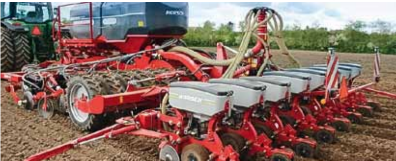
Focus TD with three-point linkage and a Maestro RC seed unit bar
