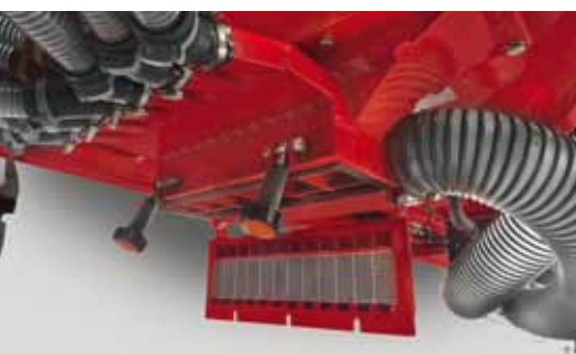
Open Seed on Demand system at the Maestro SW
