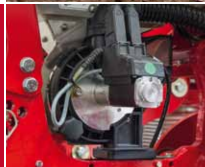
Compact and robust – the Maestro single grain metering device
