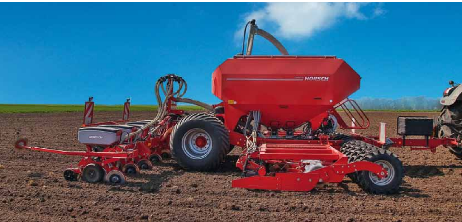
Maestro RC: Maestro seed bar (8- or 12-row) combined with seed wagon SW 3500 of the Pronto AS. The Pronto seedbar can be replaced with the Maestro seedbar and vice versa via a three-point.
