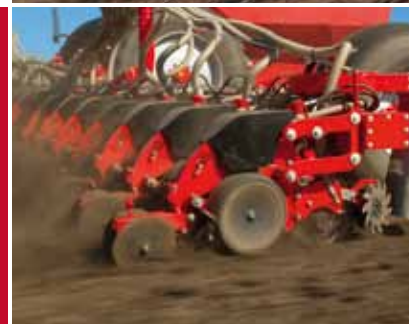
Extremely robust single grain seed units with precise grain singling and Seed on Demand system
