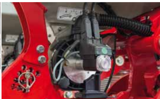
The patented metering system is unique (date 09.2011) and combines singling, engine and control unit in one casing.
