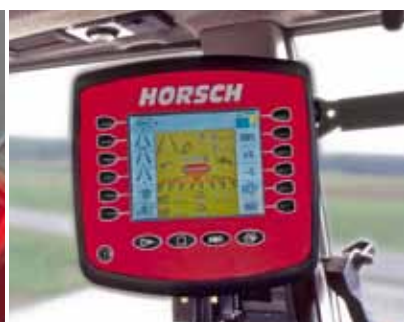
ISOBUS Terminal for checking and controlling the functions of the machine.
