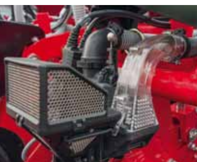
Metering unit in the Seed on Demand version
