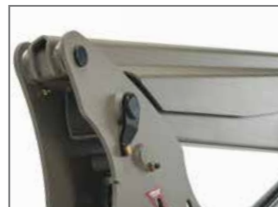
Large pivot pins with anti-rotation system for maximum durability.
