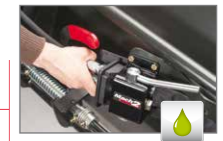
Instant connection of loader to implement hydraulic lines with the MACH 2 System®.
