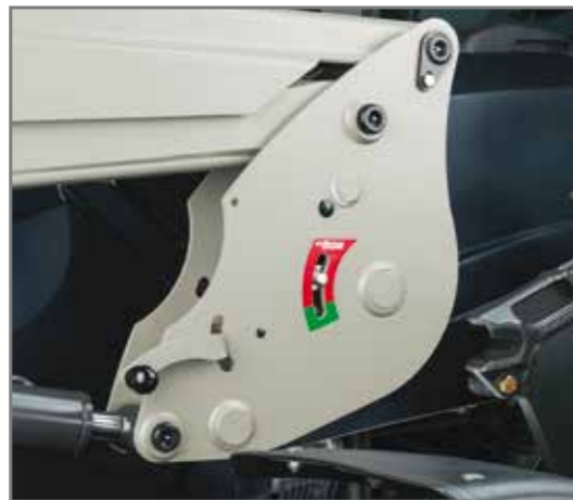
FITLOCK System® for easy drive-in hitching and unhitching, requiring only one exit from the cab.
