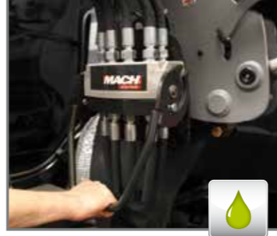
MACH System® - "non drip" instant coupling of tractor to loader hydraulic and electric lines.
