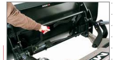
Automatic locking implement carrier: Well positioned release handle.
