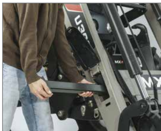
Protected parking stands integrated into the loader crossbar: Loader lift clearance is not compromised.
