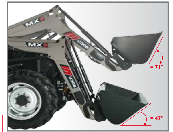
Crowding angle offering maximum efficiency: up to 71° at 1.20 m from the ground.
