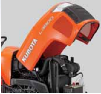
Slide-out radiator screen / Gas-strut open hood
