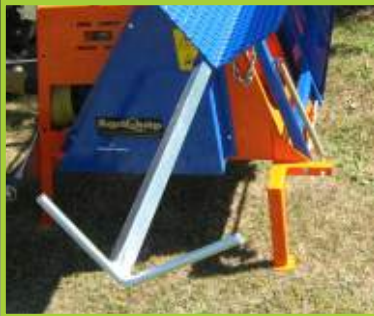
support arm for longer logs (R700)
