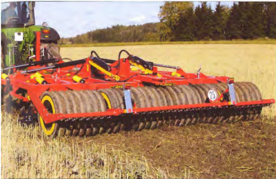
Cultus has different equipment possibilities depending on if it shall run on light or heavy soil. Heavy soil shits combined with a steel roller gives it strong power on heavy soil. On lighter soil the rubber roller is suitable combined with the light soil shits.
