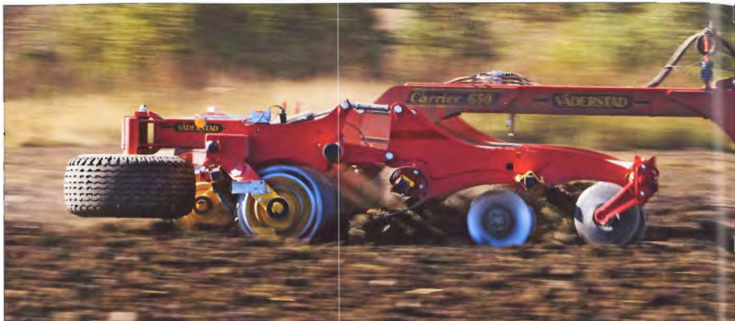
After ploughing Carrier work the clods. By choosing a Carrier equipped with a Crossboard, you get even more cultivation power. The Crossboard is available on models with up to 6.5 m working width.
