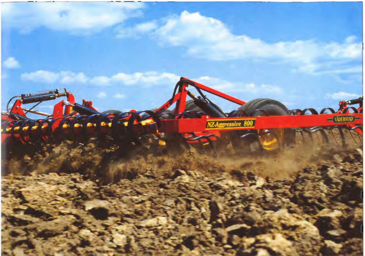
After ploughing NZA levels the field and works the soil well to produce a good seedbed.
