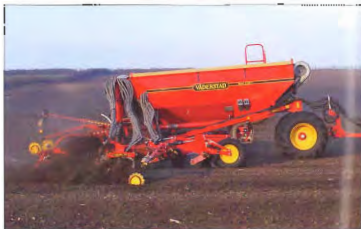
the soil after placing the seed, which means that several passes can be saved. This saves both time, fuel and soil moisture.
