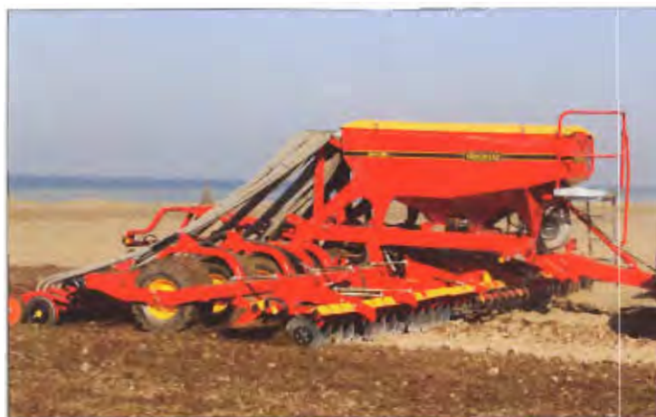
Both Spirit and Rapid have a strong cultivation ability, and perform a final cultivation before placing the seed. The drill also consolidates
