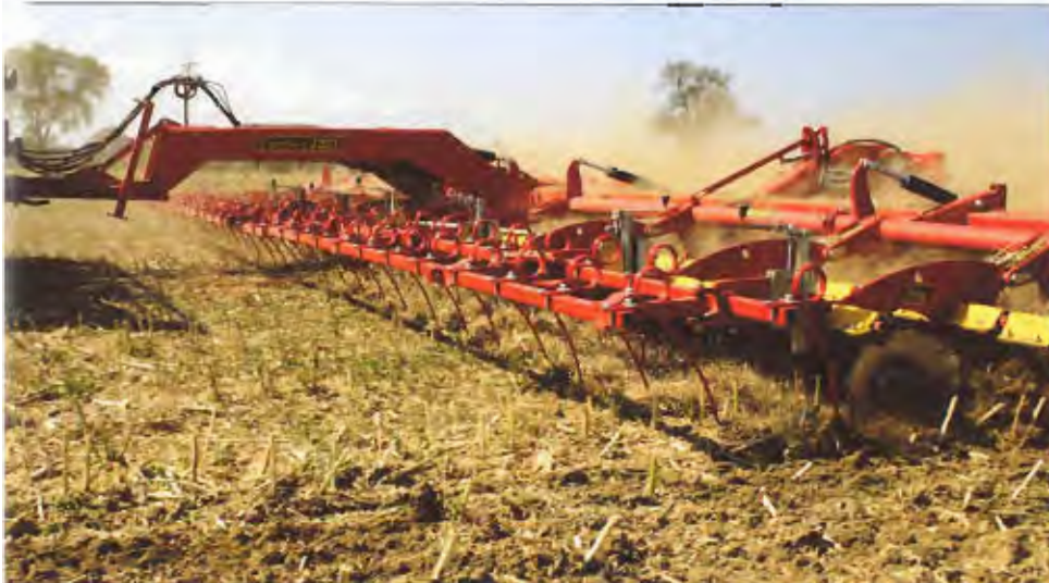
In deep cultivation without plough, the straw management is very important. With a straw harrow on the Carrier, the straw is distributed once more before cultivation.
