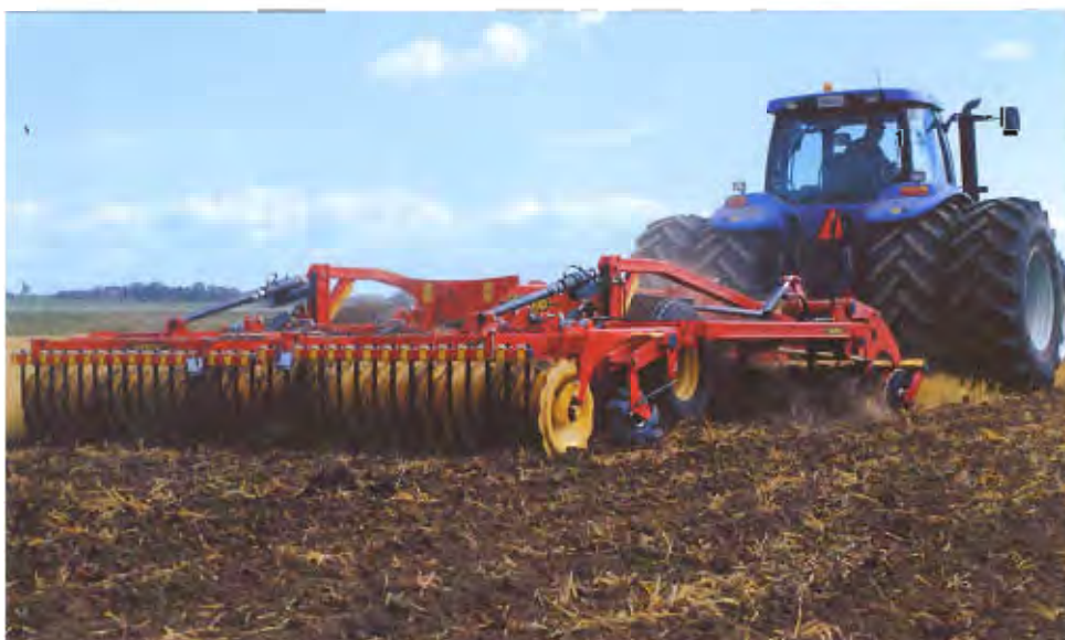
TopDana is a multi cultivator with high capacity. The working depth can be varied between 1 to 25 cm.
