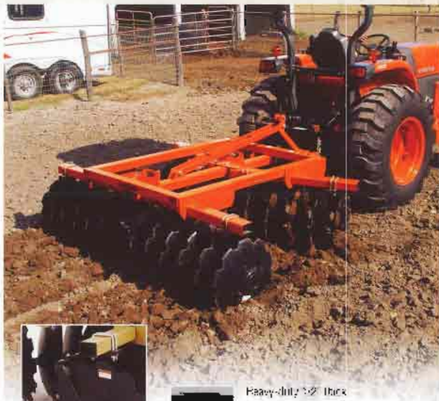
Disc scrapers are available to reduce build-up on discs.
