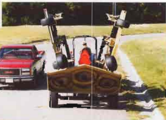
Transport width of 9' 8" allows for safe transport from site to site.
